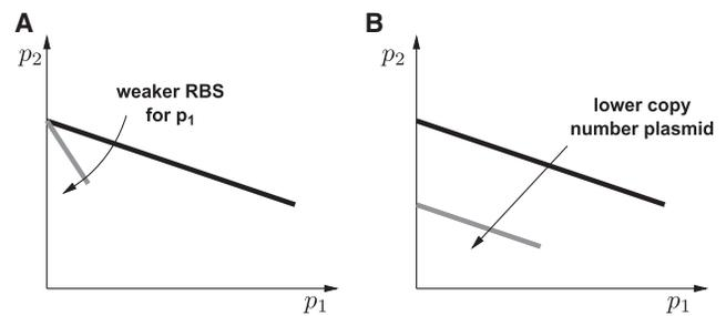
FIGURE 2 Isocost lines predicted by the model. (A) Decreasing the RBS strength of RFP ( $p_1$ ), that is, increasing the dissociation constant  $k_1$ , rotates the isocost line clockwise. (B) Decreasing the plasmid copy number  $n$  shifts the isocost line down.
